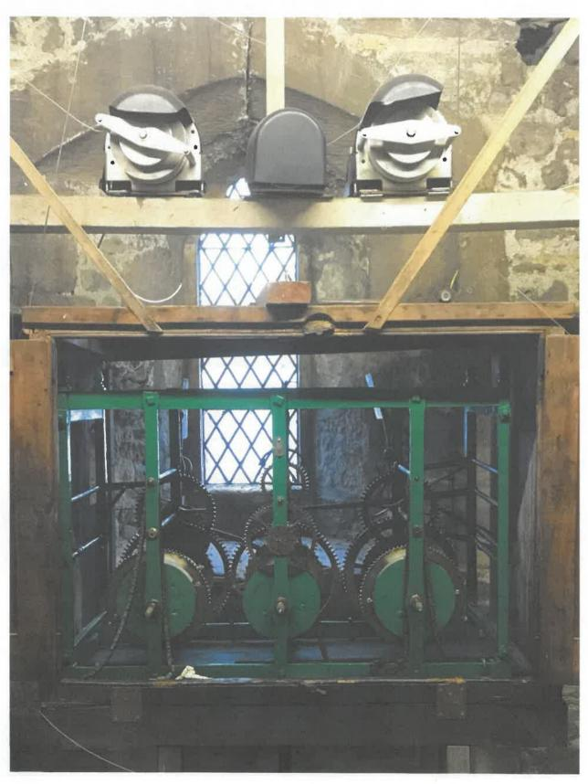
The clock will need to be repositioned, the mechanism adjusted, and the towns historic bells reconnected.
